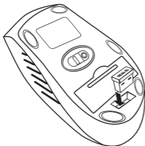
Fig. 6. Fitting the receiver into the mouse case
